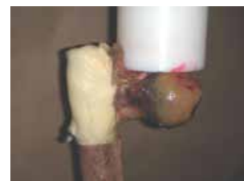
Figure 5: This specimen failed when the proximal screw cut out through the femoral head.
