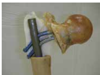
Figure 6: This specimen failed by proximal screw bending.
