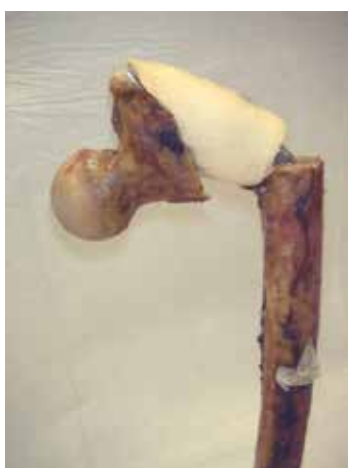
Figure 7: This specimen failed by nail bending.
