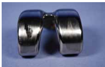
Figure 2: Severe femoral component damage
